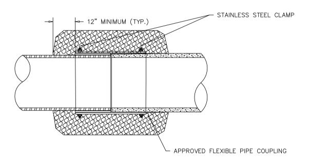
NOTE: ONLY ONE TRANSITION IN PIPE MATERIALS ALLOWED BETWEEN ANY TWO MANHOLES
